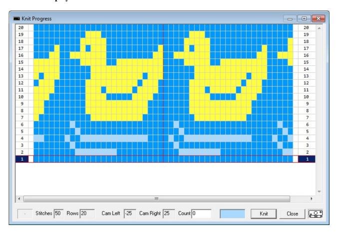
Your computer screen displays the stitches to be knitted and the progress of your knitting. You can select with a single click the row where you want to start knitting. The full screen of your computer can be used to display your pattern as it will be knitted. A row counter, point cam placement, carriage position and contrast color indication are displayed too.
